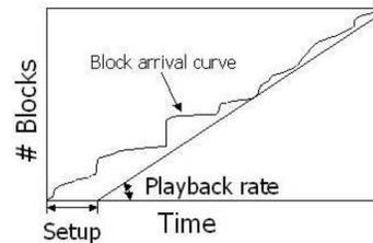
Figure 1: This hypothetical graph shows the calculation of sustainable playback rate, given the setup time. The y-axis shows the number of consecutive blocks, while the x-axis shows the time.
